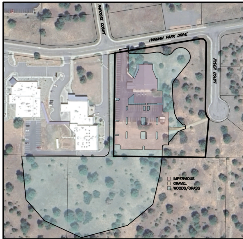
Figure 4 – Developed drainage basin configuration.
